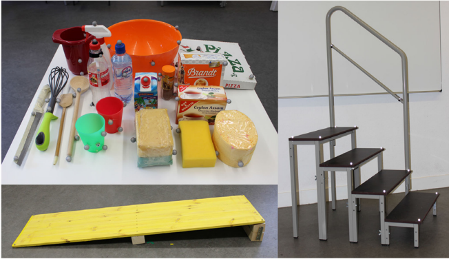
Fig. 6. Exemplary environmental elements and objects with markers attached to them for simultaneous capturing of subject and object motion.
